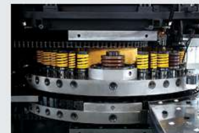
厚转塔结构 Thick turret structure 采用球墨铸铁、长镶套式结构, 延长使用寿命 It is of spheroidal graphite cast iron and long-bushing structure for long service life.
